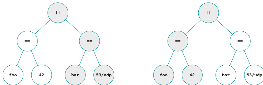
Figure 3.10: Candidate check optimization. Consider the two events foo = count and bar = int , and the query expression foo == 42 || bar == 53/udp . For event foo , the candidate checker prunes the right half of the tree (left AST), and for event bar the left half (right AST). This minimizes the candidate check operations per event.
