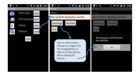
Figure 5.5: Operation of the DTN application for publishing content (photo or video file)
