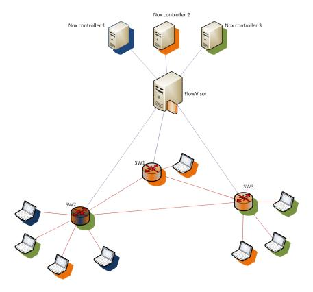
Figure 4.1: Slicing schema over the DC infrastructure
