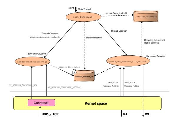
Figure 3.5: Mobile Node software architecture
