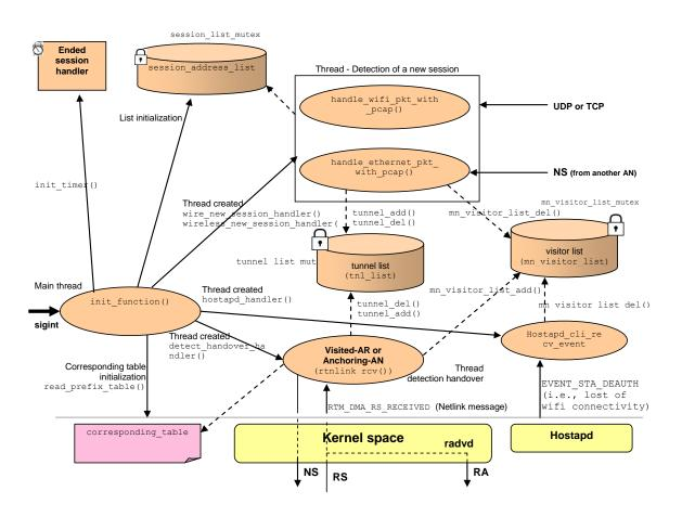
Figure 3.4: Access Router software architecture
