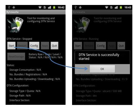
Figure 5.3: Launching the DTN service operation for Android: initial screen of Bytewalla
