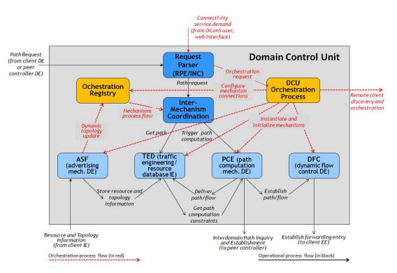
Figure 4.7: Domain control architecture - realization of internal DCU modules
