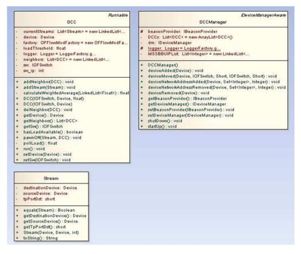
Figure 4.13: UML specification of DCC ClassObjects
