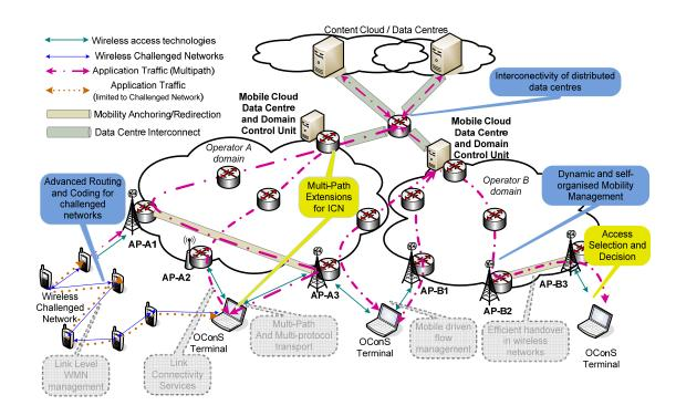
Figure 2.1: Selected OConS Architectural Components and Mechanisms for Prototyping and Demonstrations
