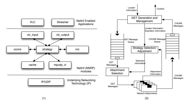
Figure 5.1: (1) OConS Multi-path Enabled NetInf Node Architecture (2) Splitting Strategy Algorithm
