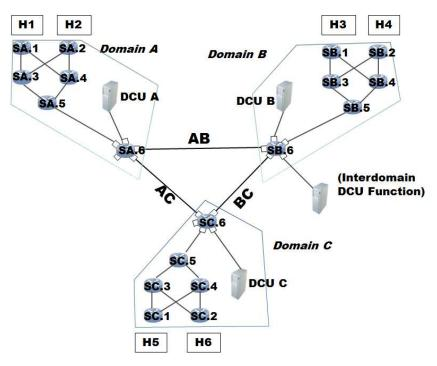
Figure 4.8: Network topology of the lab test-bed with 3 domains with labels A,B,C – 'H': denoting hosts, 'S': denoting switches
