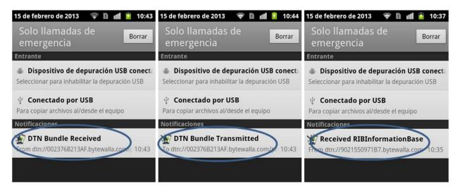
Figure 5.4: Notification of DTN routing information exchanged via HURRy protocol
