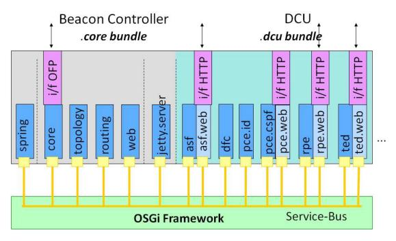
Figure 4.9: OSGi-based SW Architecture of the DCU
