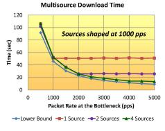
Download of a 50 MB file from 1/2/4 sources shaped at 1000 pps each, 2 hops, with a network bottleneck at 500→5000 pps
