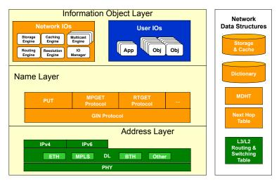
Figure 2.34: Protocol stack of the GIN Architecture
