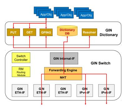
Figure 2.32: GIN prototype architecture
