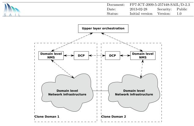
Figure 6.3: CloNe domains and the Distributed Control Plane (DCP)
