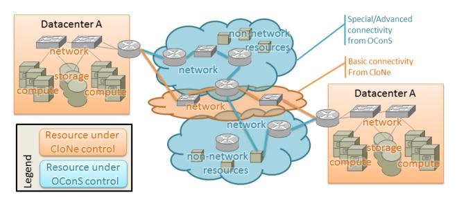
Figure 6.2: Distribution of control between CloNe and OConS. Inside Datacenters CloNe is in charge of resource control. Between Datacenters two options exist: Either (i) the special connectivity services of OConS are used, or (ii) CloNe network operators provide and manage basic connectivity.
