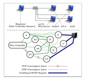
Figure 4.3: Sample NetInf multi-source network setup
