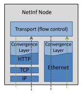
Figure 4.2: NetInf Transport protocol stack
