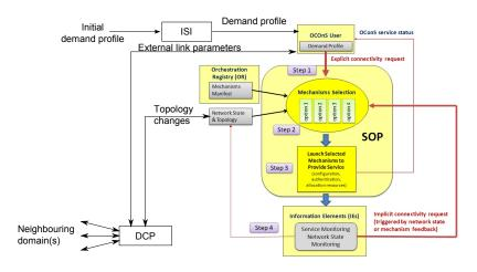
Figure 5.2: A simple integration of the CloNe interfaces with the OConS Service Orchestration Process
