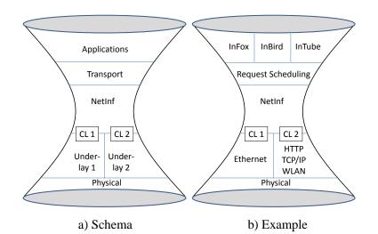
Figure 4.1: NetInf protocol stack, assuming a node with two convergence layers over two different underlays
