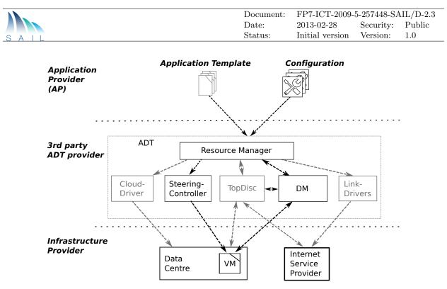
Figure 3.3: The detailed ADT architecture
