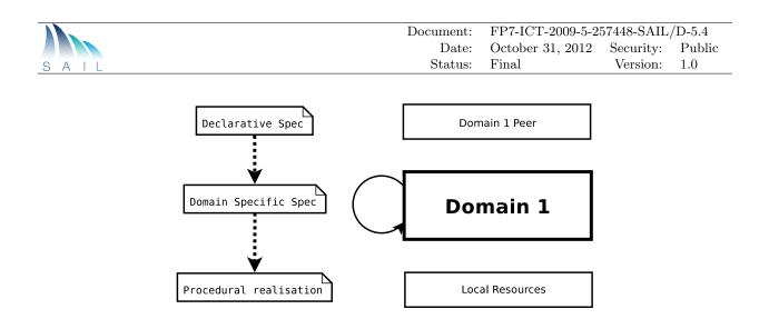
Figure 5.1: Concretisation of the high level declarative model specification into procedural domain and technology specifications
