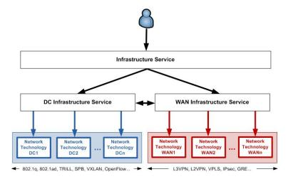
Figure 3.1: Separation of technology-independent and technology-dependent functions
