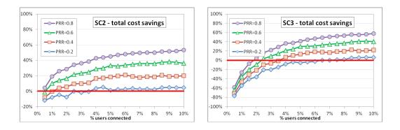
Figure 4.34: Relative savings from Caching for SC2 (left) and SC3 (right) deployment scenarios, as a function of number of connected users
