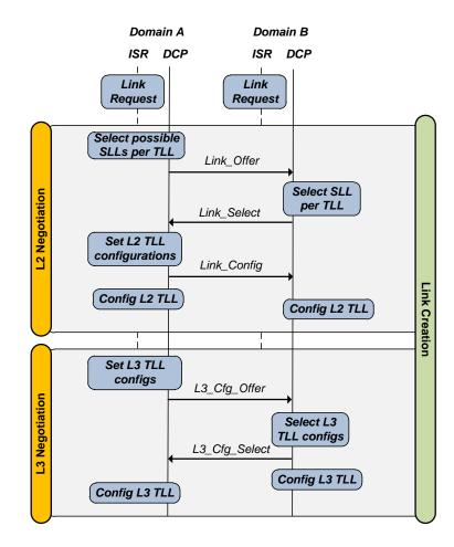
Figure 4.8: Creation Function - sequence diagram
