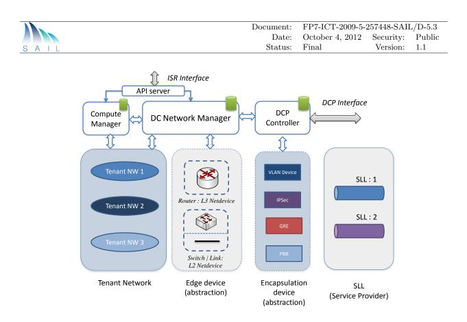
Figure 4.12: Components involved in the link negotiation and setup process in a DC domain
