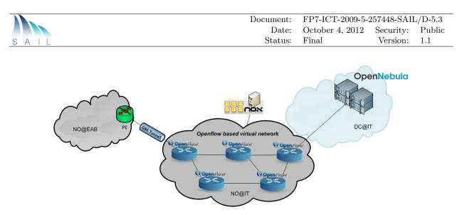
Figure 3.6: IT - OpenFlow network test bed
