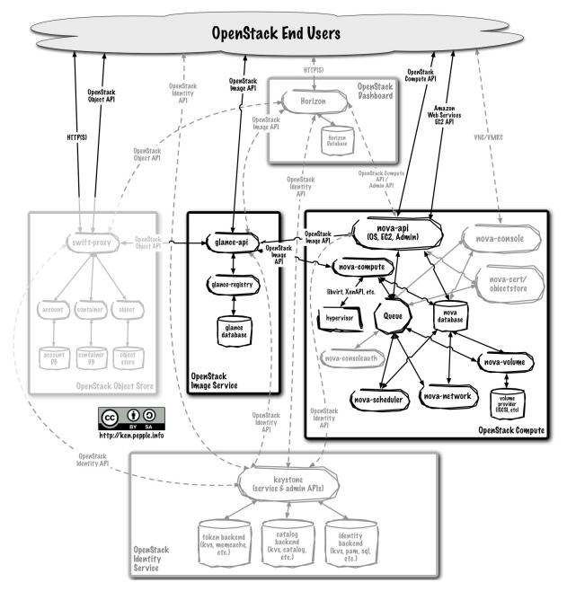
Figure 3.1: Flow between OpenStack Services
