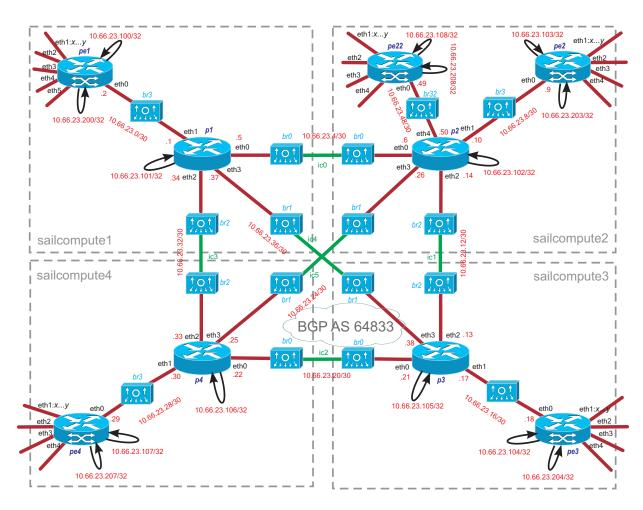
Figure 3.5: Ericsson WAN Testbed - IP/MPLS Network
