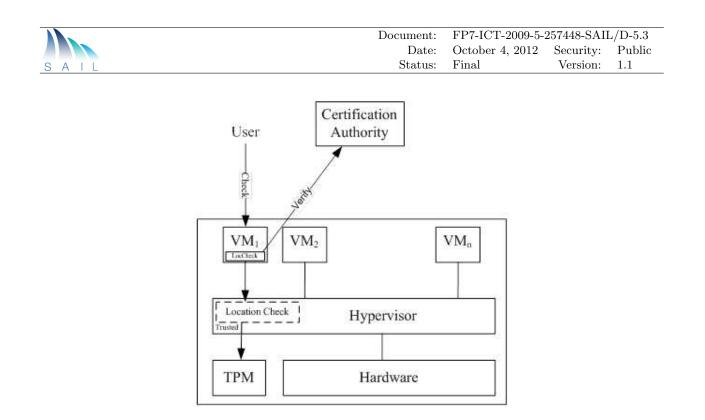
Figure 6.3: Setting for TPM-based Geo-positioning
