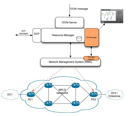
Figure 4.15: Components involved in FNS management in IP/MPLS NO domain
