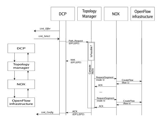
Figure 4.17: Integration of NOX OpenFlow Controller with DCP - Establishing a network path
