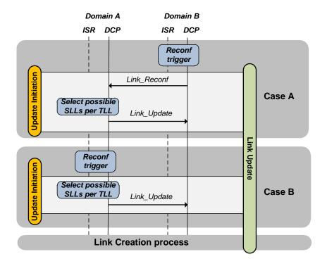
Figure 4.9: Update Function - sequence diagram
