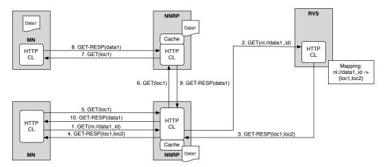
Figure 5.5: Example of how MN queries the published content from infrastructure service (RVS) to get the locator and then retrieves the NDO from the publishing MN.
