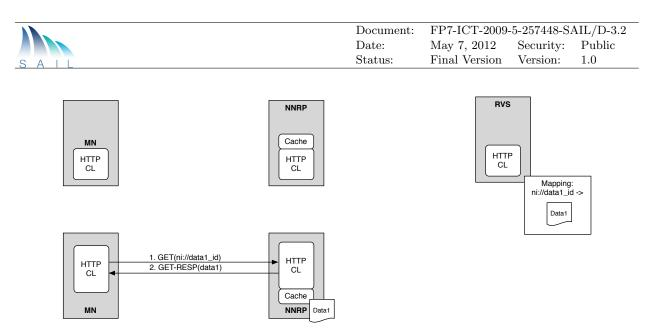
Figure 5.3: Example of how MN queries the published content that is cached in NNRP from in-frastructure service (RVS).
