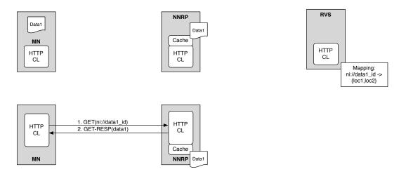
Figure 5.6: Example of how MN queries the published content that is cached in NNRP and that is directly served from there.
