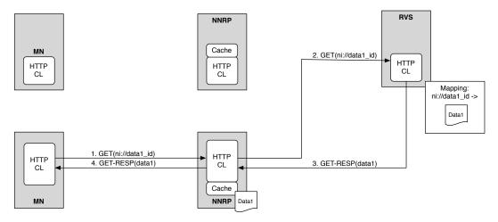
Figure 5.2: Example of how MN queries the published content from infrastructure service (RVS).
