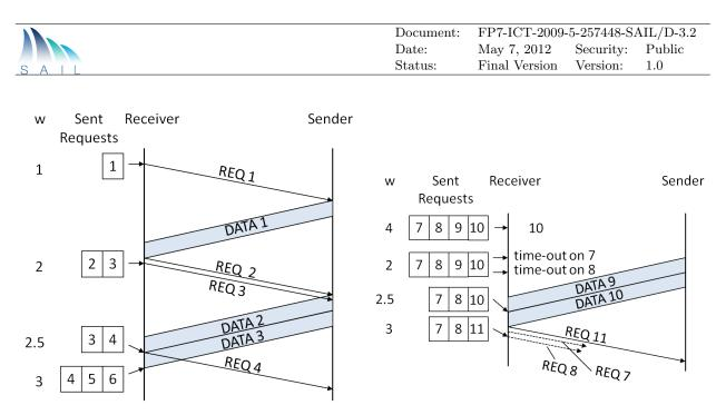
Figure 3.3: Trellis diagram for window evolution: increase (left), decrease (right).
