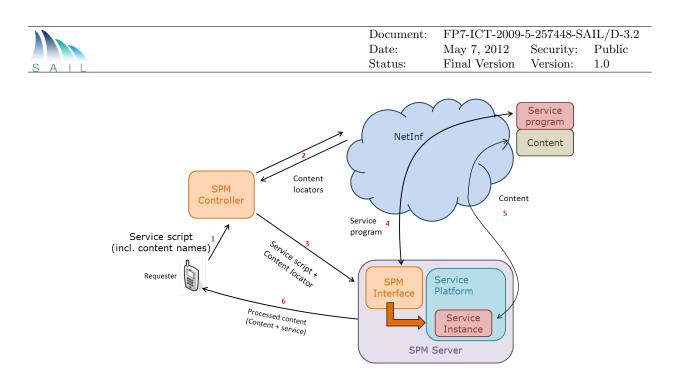
Figure 4.1: Basic SPM Architecture and Functionality.
