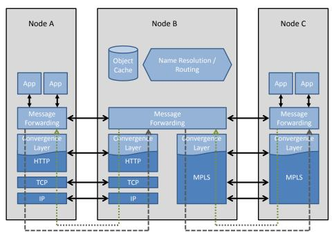
Figure 2.1: Example NetInf Convergence Layers
