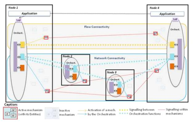
Figure III: Example of OConS network model, illustrating the orchestration functionality.
