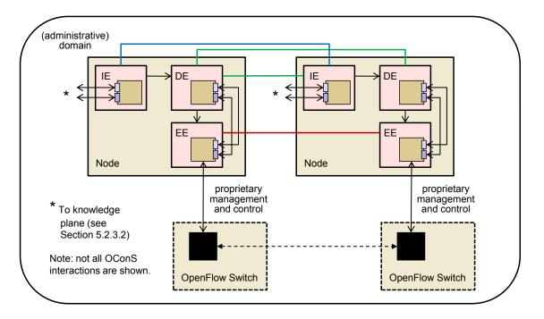
Figure 5.5: Management in the OConS architecture, based on Figure 4.2 in [3]. Not all OConS interactions are shown, for colour codes see Figure 4.2 in [3]. For symbols, refer to Figure 5.4.
