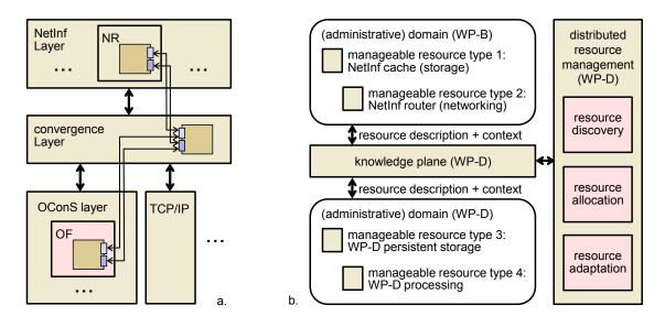
Figure 5.7: Inter-WP management interactions. — a. Management across layers, based on Figure 3.5 in [2] and Figure 4.2 in [3] (NR: NetInf router; OF: orchestration function (OConS)).
