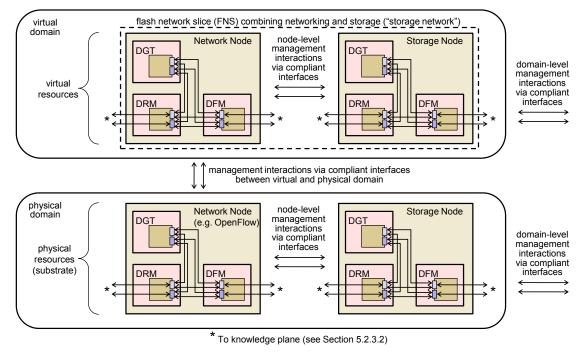
Figure 5.6: Management in the CloNe architecture, based on Figure 2.4 and 4.4 in [4]. The figure shows only an exemplary setup in the peer-to-peer interaction case, among many other possibilities.
