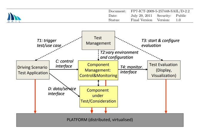
Figure 3.3: Prototyping, Test and Experimentation Framework
