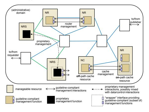
Figure 5.4: Management in the NetInf architecture, based on Figure 3.2 and 3.3 in [2].
