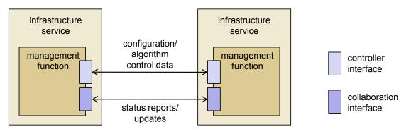
Figure 3.2: Interaction between management functions via WP-D's two types of interfaces.
