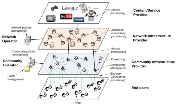
Figure 15: Actors and roles of the Wireless Challenged Networks use case
