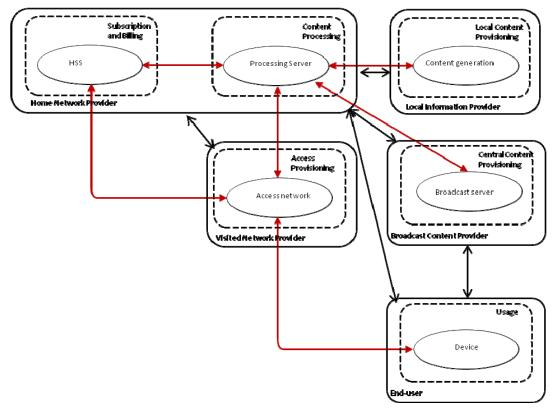
Figure 11: Current architecture without NetInf
