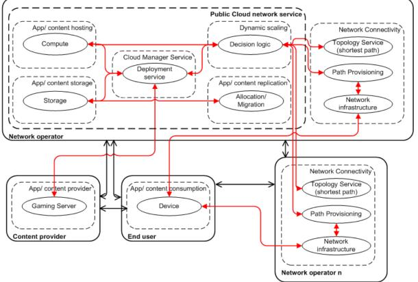
Figure 25: Industry and technical architecture for the Distributed Gaming use case
