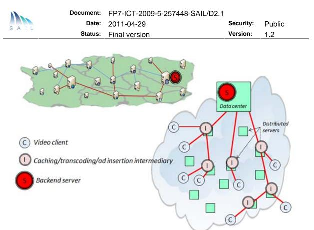
Figure 23: Distributed Cloud architecture concept illustration for Live Video Distribution
