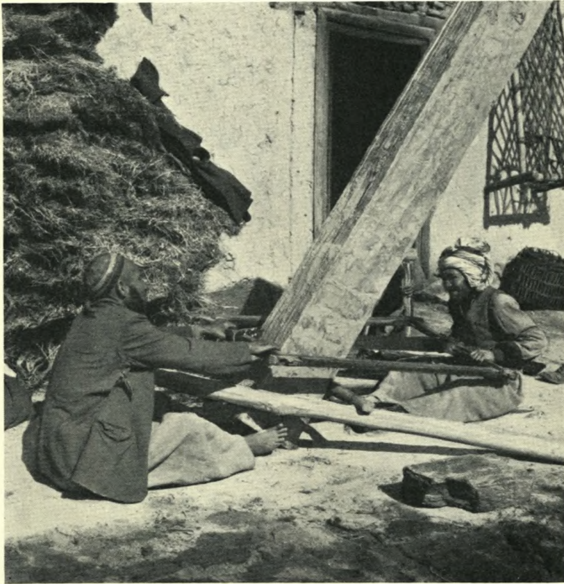
Fig. 13. Hazāra labourers in a street in Kābul sawing up a plank into boards (Spring 1954 by K. F.).
