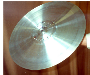
Front and back views of one of the chopper disks. The white material is Gd 2 O 3 , which is a very strong neutron absorber. Neutrons pass through the wedge-shaped bare metal areas.
