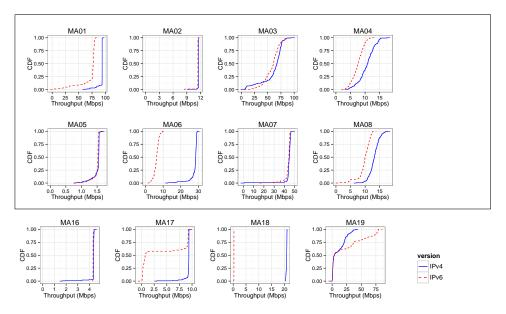
**Fig. 7.** *Distribution of line rates observed by probes wired in behind a residential gateway (boxed) and operator's lab network (unboxed). Line rates are measured using speed test against dual-stacked M-Lab servers.*
