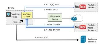
Fig. 1. A measurement setup on top of the SamKnows platform. A dual-stacked probe in addition to the standard SamKnows tests, executes the YouTube test. The YouTube test runs every hour and measures a set of performance indicators to endpoints delivering YouTube audio and video both over IPv4 and IPv6. The locally collected measurement results are pushed every hour to the SamKnows data collection server using HTTP.
