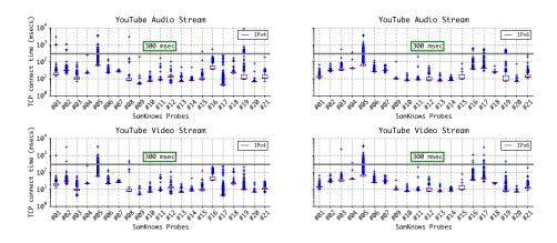
**Fig. 4.** Boxplots of TCP connection establishment times (in log-scale) to YouTube audio (above) and video (below) streams from each vantage point both over IPv4 (left) and IPv6 (right). The raw TCP connect times to YouTube media servers are comparable over both address family.
