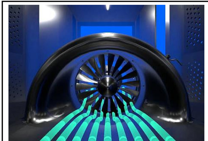
The Boundary Layer Ingestion (BLI) Inlet Distortion Tolerant Fan (DTF) installed in NASA GRC's 8'x6' wind tunnel, a new capability to investigate fuel burn reduction potential by embedding an aircraft's engine at the rear of an aircraft compared to an under the wing conventional configuration.
