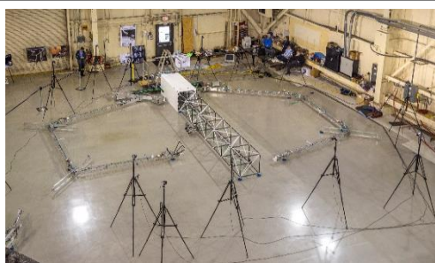
Innovative NASA robotic technologies such as TALISMAN, seen here during calibration tests at NASA's Langley Research Center, are critical to the CIRAS project, which seeks to enable space-based, robotic assembly of flight hardware and space systems. This is one of three concepts being developed.
