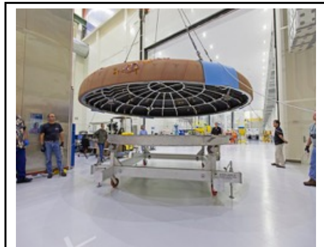
October 23, 2017 Orion heat shield for EM-1 moves toward the thermal chamber in Neil Armstrong Operations and Checkout building at NASA's KSC in Florida. It will undergo a thermal cycle test to verify acceptable workmanship and material quality.
