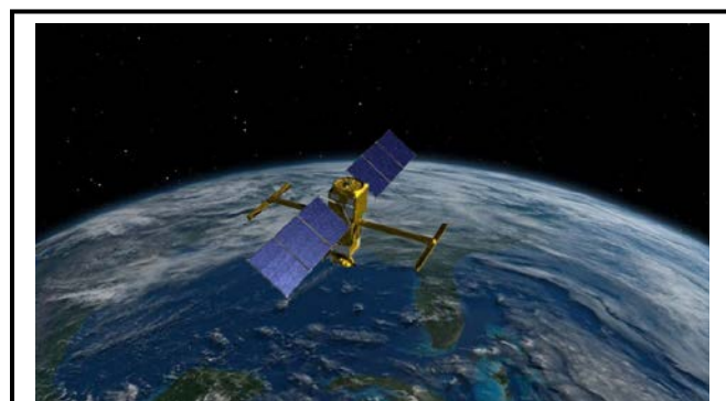
An artist's conception shows the Surface Water Ocean Topography (SWOT) satellite, which entered the implementation phase in May 2016. SWOT will make high-resolution, wide-swath altimetric measurements of the world's oceans and fresh water bodies to understand their circulation, surface topography, and storage. This multi-disciplinary, cooperative international mission will produce science and data products that will allow for fundamental advances in the understanding of the global water cycle.
