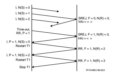
$\label{eq:FIGUREVII.5/X.25} I \ frame\ recovery,\ when\ multiple\ I\ frames,\ last\ I\ frame\ and\ SREJ\ frames\ are\ lost$
