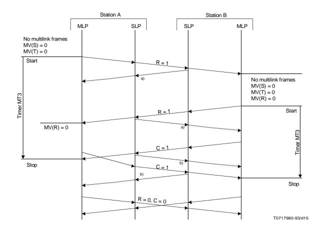
a) The SLP frame that acknowledges delivery of the multilink frame with R = 1.
