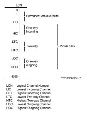
Logical channels 1 to LIC-1: Range of logical channels which may be assigned permanent virtual circuits. Logical channels LIC to HIC: Range of logical channels which are assigned to one-way incoming logical channels for virtual calls (see 6.8).
