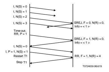
$\label{eq:FIGUREVII.2/X.25} I \mbox{ frame recovery, when SREJ frame with F bit set to 0 is lost}$
