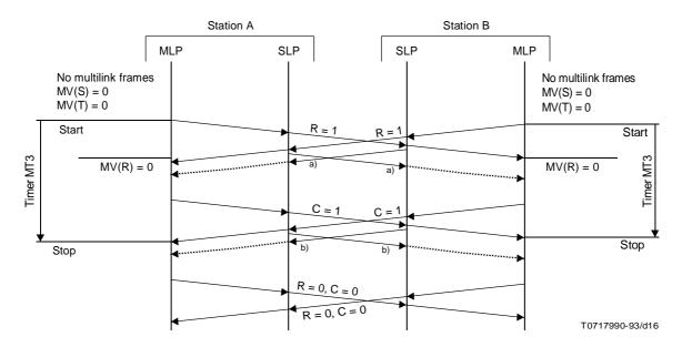
$<sup>^{</sup>a)}$  The SLP frame that acknowledges delivery of the multilink frame with R=1.
