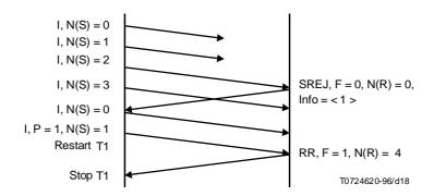
$\label{eq:FIGUREVII.1/X.25} I \mbox{ frame recovery due to SREJ frame with F bit set to 0}$
