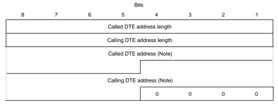
NOTE – The figure is drawn assuming the number of semi-octets present in the called DTE address field is odd and the number of semi-octets present in the calling DTE address field is even.
