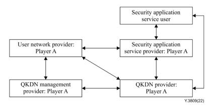
Figure 7-1 – Model 1 for QKDN based security application services
