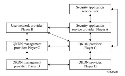
Figure 7-7 – Model 7 for QKDN based security application services
