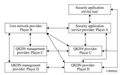
Figure 7-6 – Model 6 for QKDN based security application services
