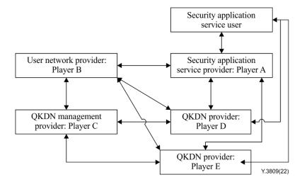
Figure 7-5 – Model 5 for QKDN based security application services
