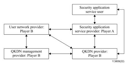
Figure 7-2 – Model 2 for QKDN based security application services
