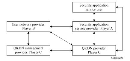
Figure 7-3 – Model 3 for QKDN based security application services
