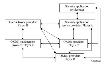
Figure 7-4 – Model 4 for QKDN based security application services
