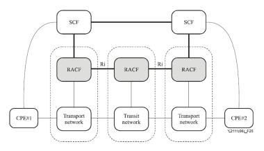
Figure 25/Y.2111 – Inter-operator RACF communications
