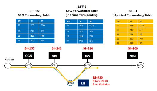
Fig-2 Heterogeneous SI assignment mechanism of SFC in mobile scenario
