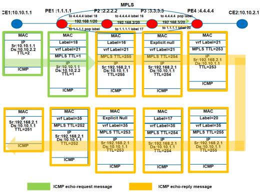
Fig 7-2 ICMP pattern of TTL=2 for End-to-End Enterprise Network Here is a simple example which explains the behavior when ICMP trace is triggered from CE1 to remote CE2 over MPLS domain:
