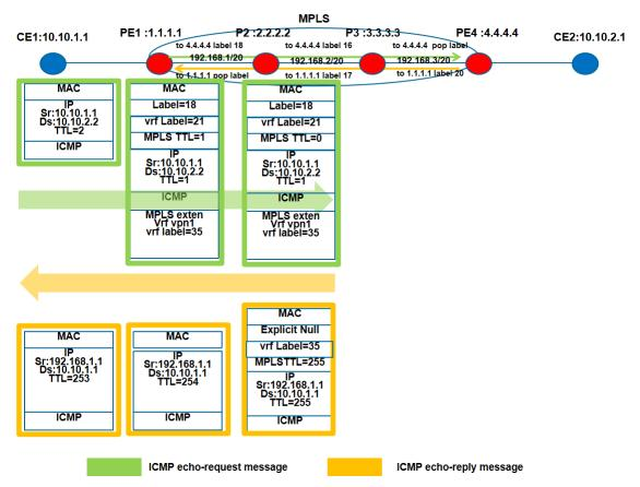
Fig 3 Optimized ICMP pattern of TTL=2 for End-to-End Enterprise Network
