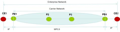
Fig 7-1 Enterprise Network through carrier's MPLS network
