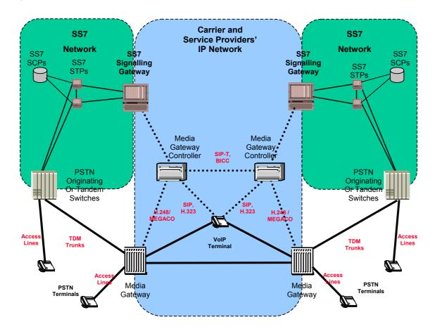
Figure 1 - ITU, IETF & ETSI VolP Architecture for Carriers and Service providers
