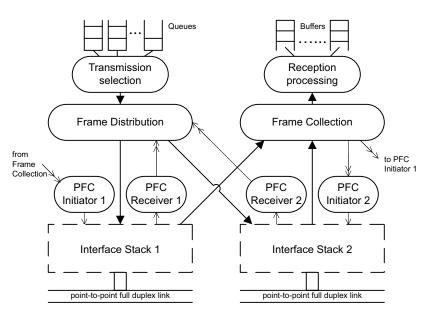
Figure 36-12—PFC operation with link aggregation
