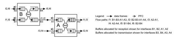
Figure 36-6—PFC congestion spreading
