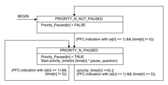
Figure 36-8—PFC Receiver state diagram for priority n
