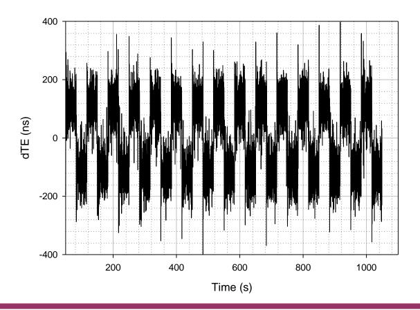
Case 1, PTP Instance (node) 90 Filtered phase offset relative to GM
