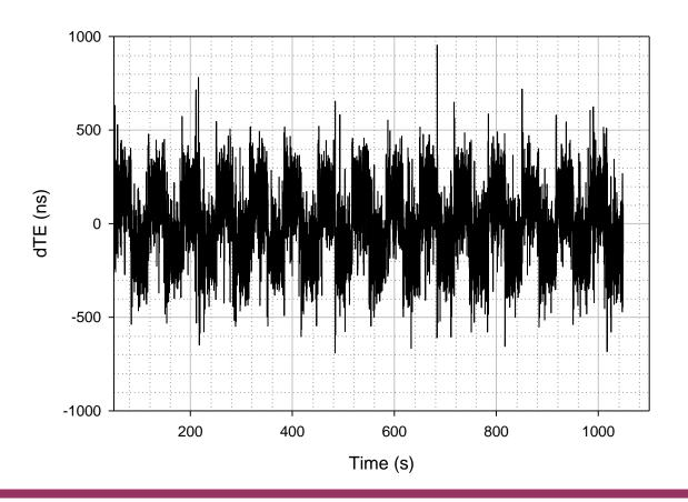
Case 1, PTP Instance (node) 100 Filtered phase offset relative to GM
