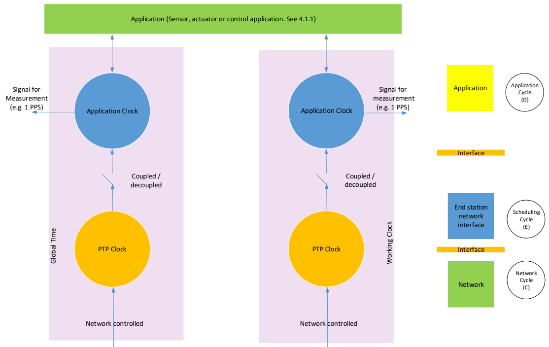
Figure 15a: Alternative clock usage model
