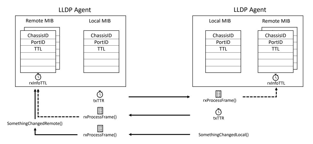
NOTE: Think of the Remote and Local MIBs as a database that must fit into a single PDU Replace all values of the Remote MIB with contents of LLDPDU when something changes
