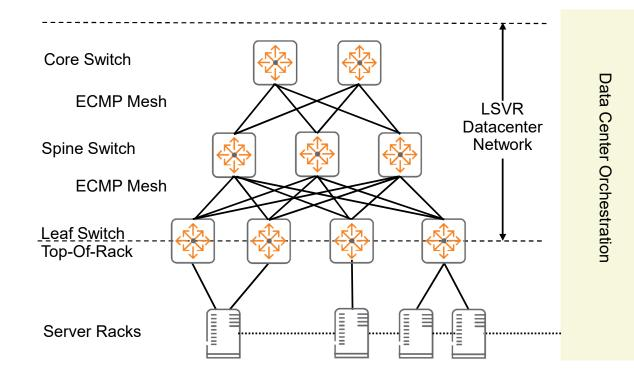
Most datacenters are configured as 2-3 layer Clos networks using ECMP for distribution over the mesh and LAGs/M-LAGs for server attachment
