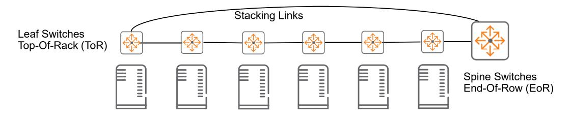
– Here the link rate between switches is lower and max hop count is higher than the Clos tree, however this is a low cost structure for a small datacenter composed of a handful of racks
