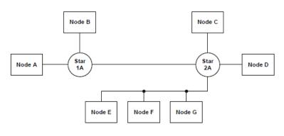
Figure 10 — Single channel hybrid example
