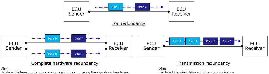
Description: The bus is duplicated and the additional lines are used to detect failures.
