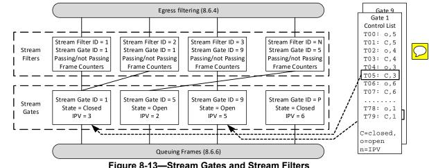
Figure 8-13—Stream Gates and Stream Filters
