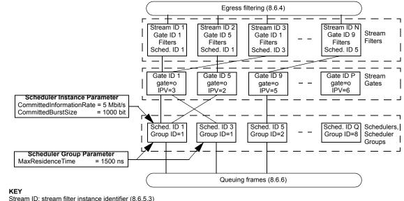
Stream ID: stream filter instance identifier (8.6.5.3) Gate ID: stream gate instance identifier (8.6.5.3, 8.6.5.5) Sched. ID:ATS scheduler instance identifier (8.6.5.3, 8.6.5.7)
