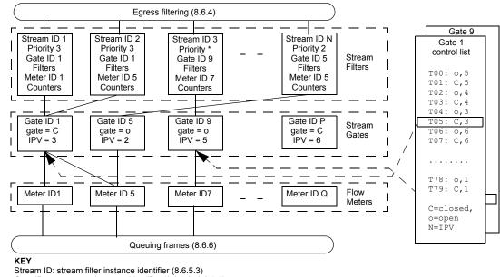
Gate ID: stream gate instance identifier (8.6.5.3, 8.6.5.5) Meter ID: flow meter instance identifier (8.6.5.3, 8.6.5.6)
