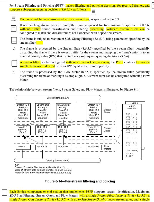
Flow Meter Instance Table (8.6.5.5) per Bridge component or end station.
