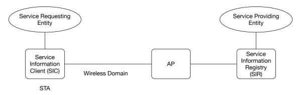
Figure 1: PAD architecture with direct communication between the AP and the SIR
