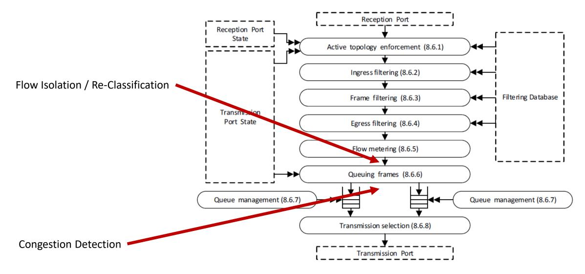
Figure 8-11—Forwarding process functions
