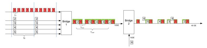
Detailed aggregation information is only required on bridges that modify/separate aggregation configuration, e.g. add or remove flows to the aggregated channel.
