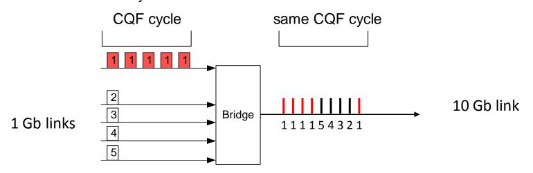
Bridging device needs to store all packets for one cycle , quite large for output port if it is x10/x100 times higher speed than input port.
