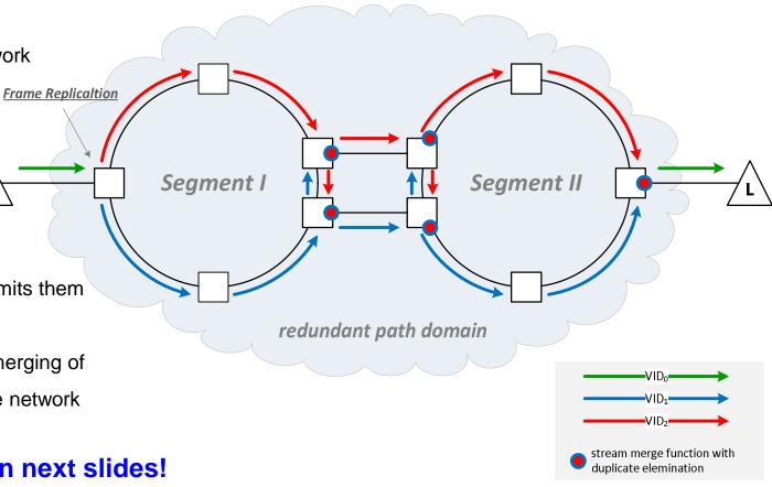
.1CB Use Case 2: Seamless Redundancy with Segment Protection Example: Ladder Redundancy with MRT
