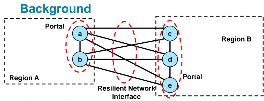
As shown in <u>new-nfinn-LACP-vs-buffer-networks-1110-v1.pdf</u>, the basic architectural blocks, control flows, and data flows for a Resilient Network Interface are largely determined by the problem requirements, independently of the choice of a particular control protocol.
