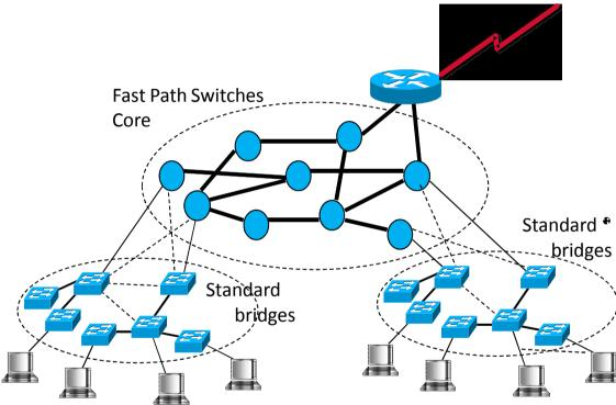
Every port detects type of connected bridge and selects working mode: STD or Fastpath (via protocol migration mechanisms) depending on its connectivity (i.e. hears FP BPDUs or not)
