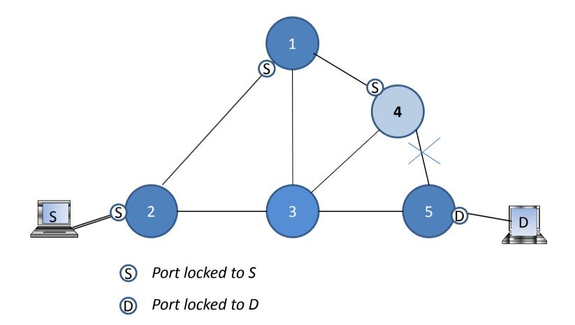
Source bridge sends ARP Request or Path Request packet to set new path
