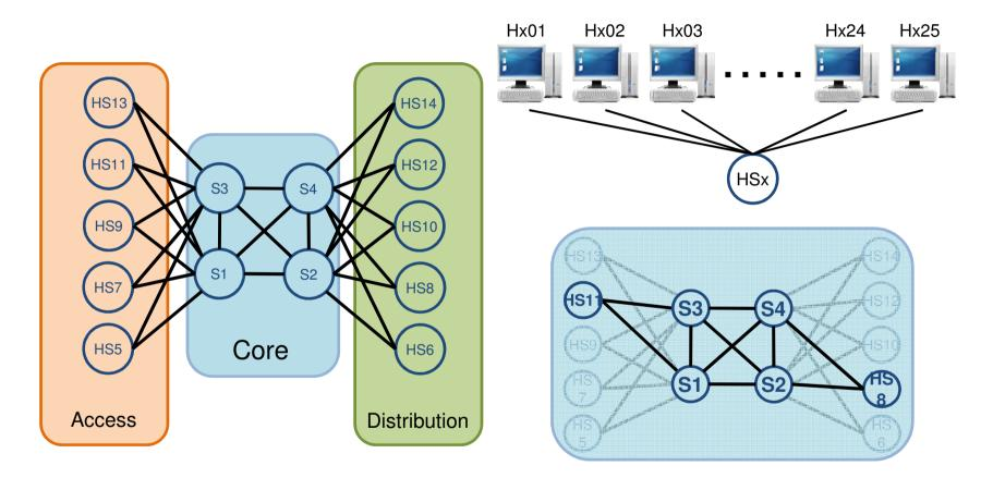
Traffic from 25 hosts connected to HS11 to 25 hosts connected to HS8. UDP of increasing length to force link loads333. All links 100 Mbps. Omnet++ simulator.
