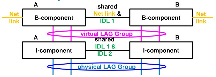
The additional DRNI between the B-components and the I-components allows the gateways to be allocated so that shared learning is not required.
