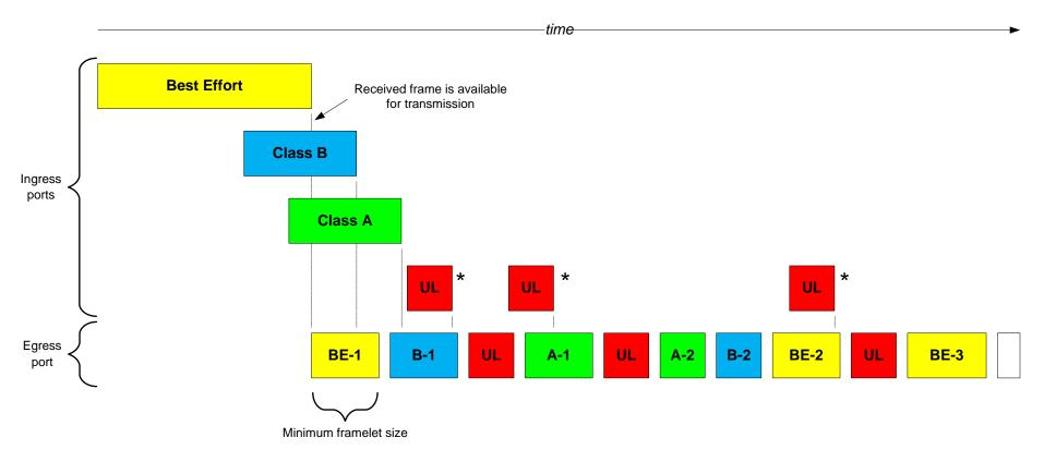
\*Note: This slide assumes Ultra-Low latency (UL) frames are separate from SR Class A & B frames
