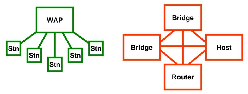
There are two very different models for "Emulated LANs": The Master/Slave model (EPON, 802.11) and the Full Mesh model (ATM LANE, VPLS).
