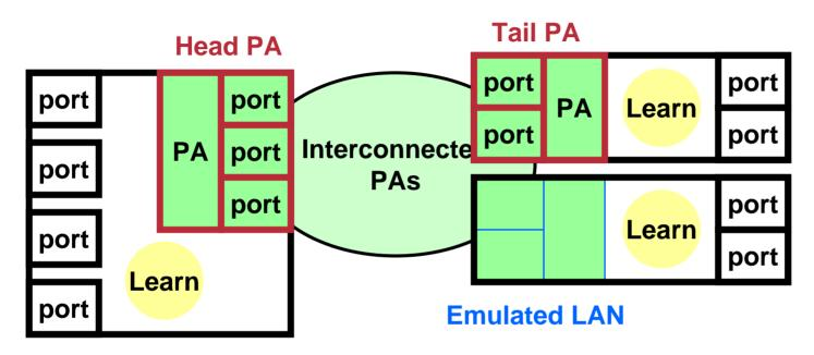
In a Bridge, a Tail PA is indistinguishable from an Emulated LAN port, because the Tail PA needs no additional Learning function.
