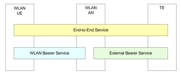
Figure 5.1 QoS Architecture for WLAN Direct IP Access
