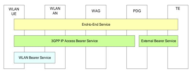
Figure 5.2 QoS Architecture for WLAN 3GPP IP Access
