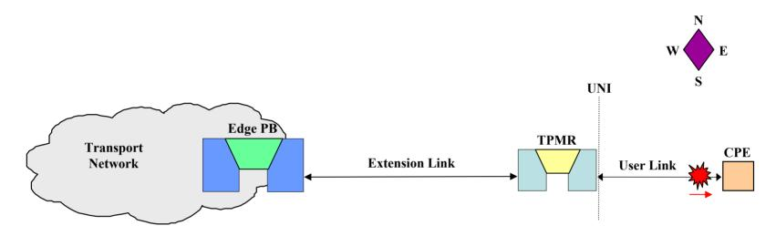
If the CPE leaves its TX on, and if Auto-Negotiation is disabled, and assuming the CPE doesn't support EFM OAM Link Fault, then no failure is detectable by the TPMR.
