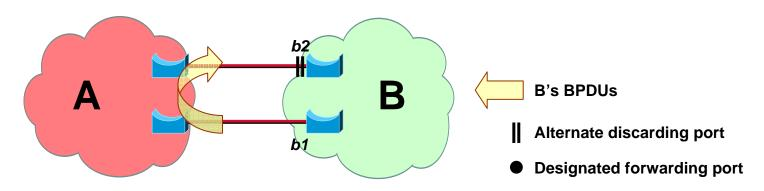
A very common solution consists in running B's STP over domain A:
