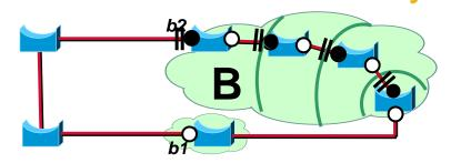
The STP sync mechanism prevents any temporary loop: the designated discarding port "travels toward" b2.
