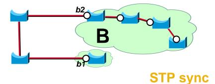
Domain B is split, *b1* and *b2* are root forwarding. A link is then brought up between the two parts.
