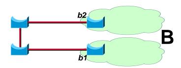
The two parts of B are connected while *b1* and *b2* are forwarding: there is a loop until the hellos from *b1* reach *b2*
