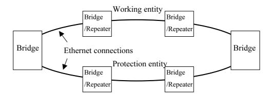
Figure 4/Y.17ethps p-p Ethernet SNC protection
