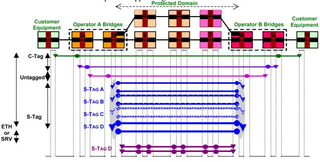
Figure 13/Y.17ethps Network model of ETH SNC/T Group Protection with Dual Relay Model with Bundling
