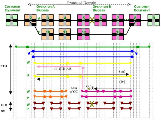
( i) ETH-CC packet of level pink does not arrive at MEP of equipment 5 for working entity, then detects Loss of CC (LOC).
