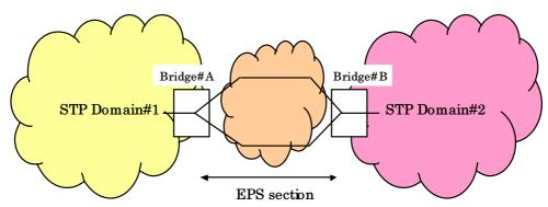
Figure II-7 Case where STP domains connected with EPS section
