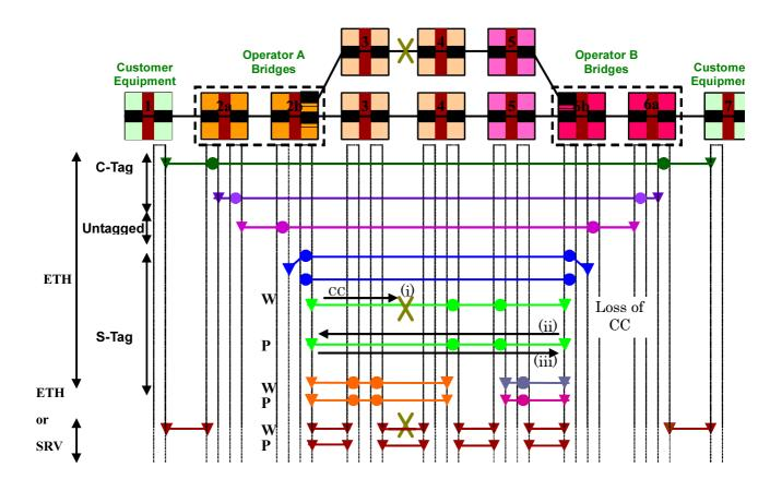
(i) ETH-CC packet of S-Tag OAM for level yellow does not arrive at MEP of equipment 6b for working entity, then detects Loss of CC (LOC).
