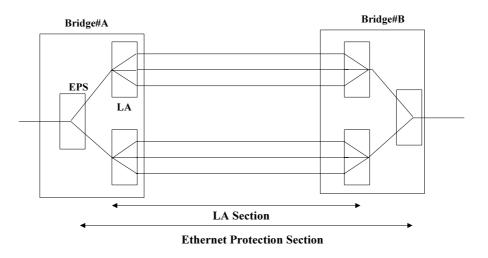
Figure I- 3 Example of LA and EPS coexisting in a bridge
