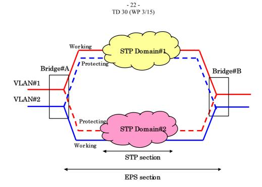
Figure A-4 Overlapping interaction between EPS and STP per VLAN
