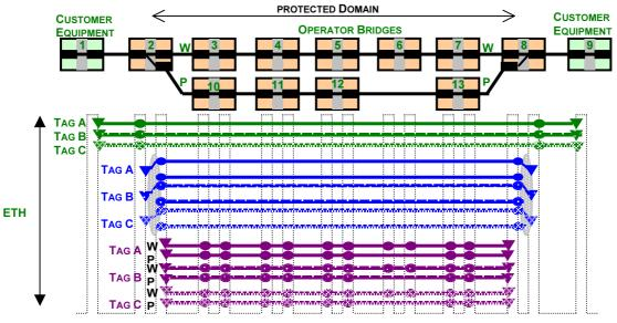
Figure 10/Y.17ethps ETH SNC/S Group Protection in single operator network
