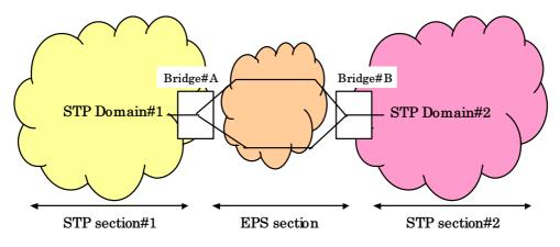
Figure A-2 No overlapping interaction between EPS and STP
