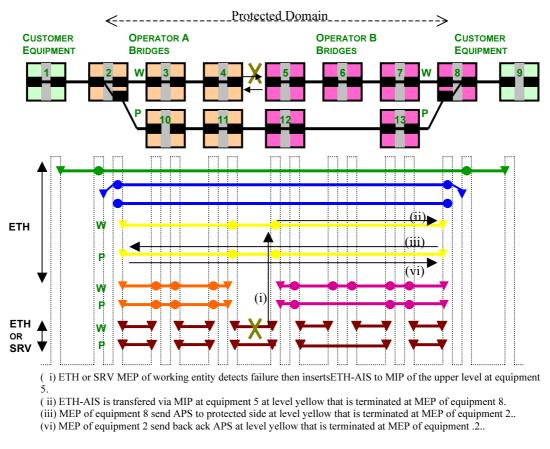
(vi) MEP of equipment 2 send back ack ETH-APS at level yellow that is terminated at MEP of equipment .2.
