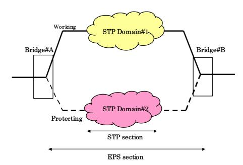
Figure A-3 Overlapping interaction between EPS and STP
