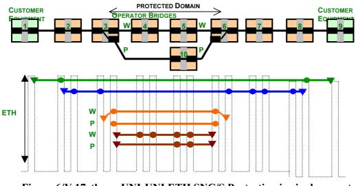
Figure 6/Y.17ethps UNI-UNI ETH SNC/S Protection in single operator network
