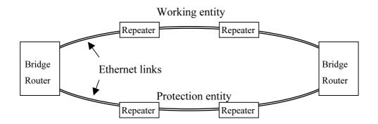
Figure 3/Y.17ethps p-p Ethernet Trail protection
