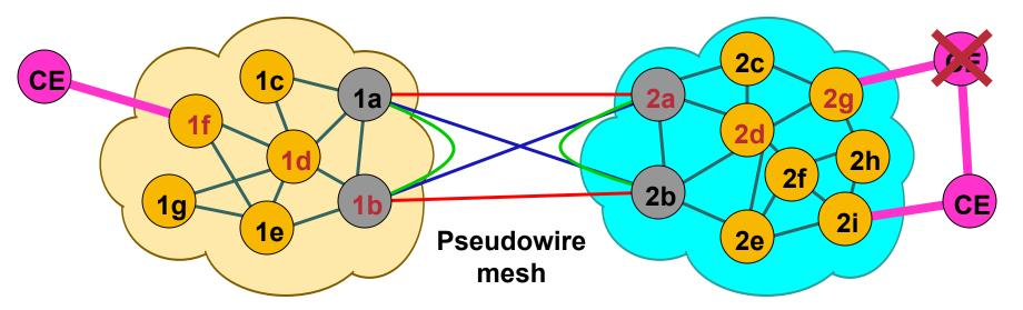
A spanning tree topology change in the Customer's network may require other Islands' bridges and LAN Emulation Forwarding Functions to forget some of that Customer's MAC addresses.
