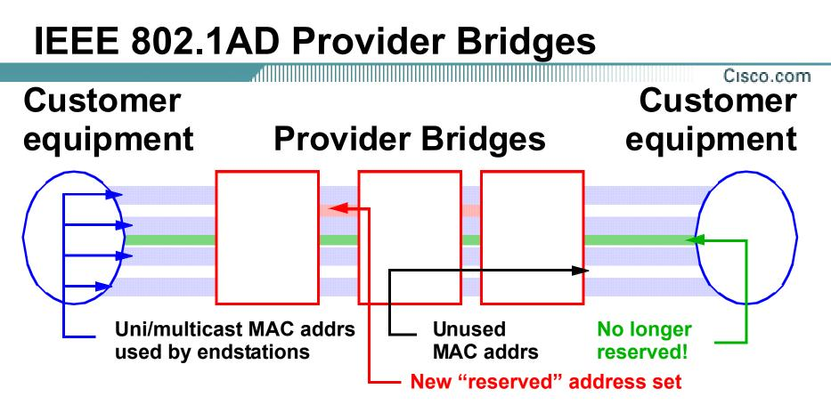
If the Provider Bridges use a new set of VLAN tags and MAC addresses, then they are transparent to Customer Equipment even if CE is a bridge!
