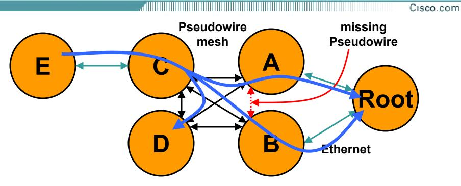
Even worse is any frame, even a normal unicast, sent from E. The frame is delivered twice to the Root.
