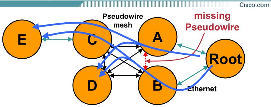
If A and B cannot see each others' BPDUs, both forward to the full mesh. C, D, and E see two copies of every multicast or unknown flood from the Root.
