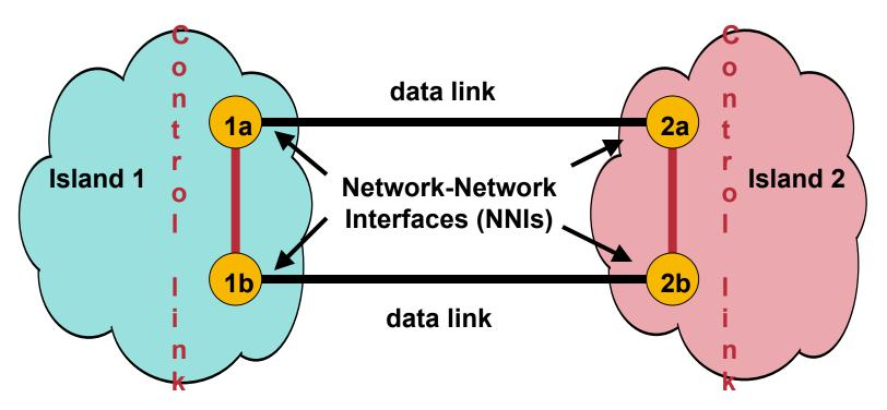
A protocol runs among the 4 Provider Bridges to ensure that only one data link is used for any given Customer Service Instance.
