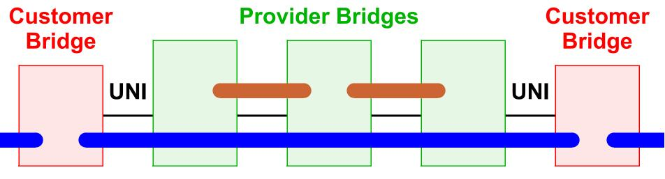
Provider addresses are peered by Provider bridges.
