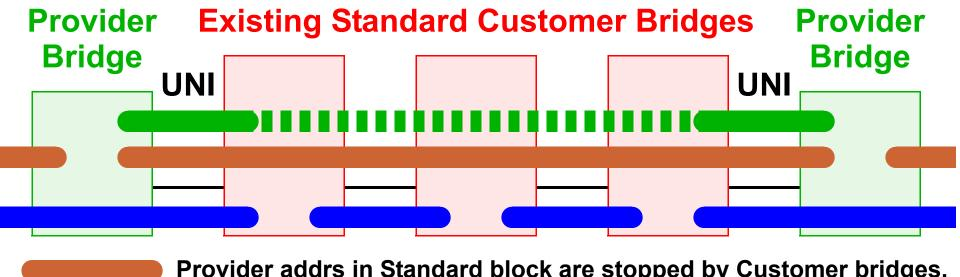
Provider addrs in Standard block are stopped by Customer bridges. Standard (customer) addresses are peered by Customer Bridges.
