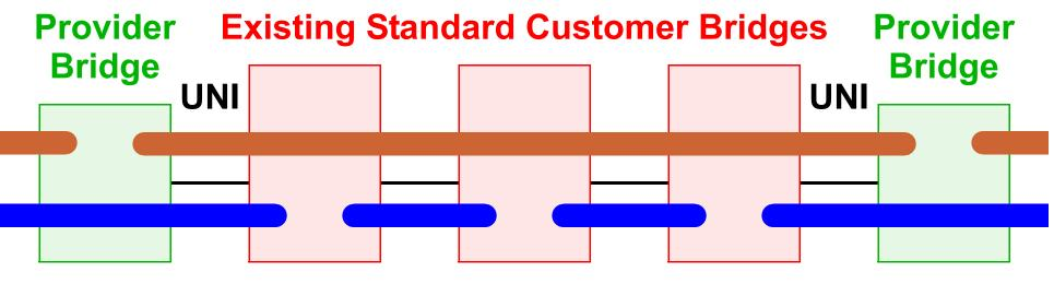
Provider addresses pass through Customer bridges.
