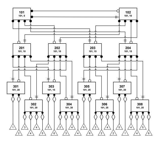
Figure 1 – Example structure provider network (part, with service VLANs 1 thru 6)
