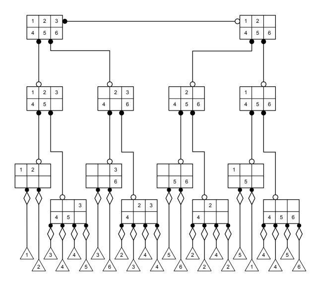
Figure 2 – Active topology of example structured network with VLANs
