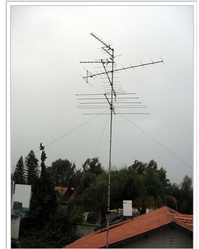
Rooftop television antennas. Yagi-Uda antennas like these six are widely used at VHF and UHF frequencies.
