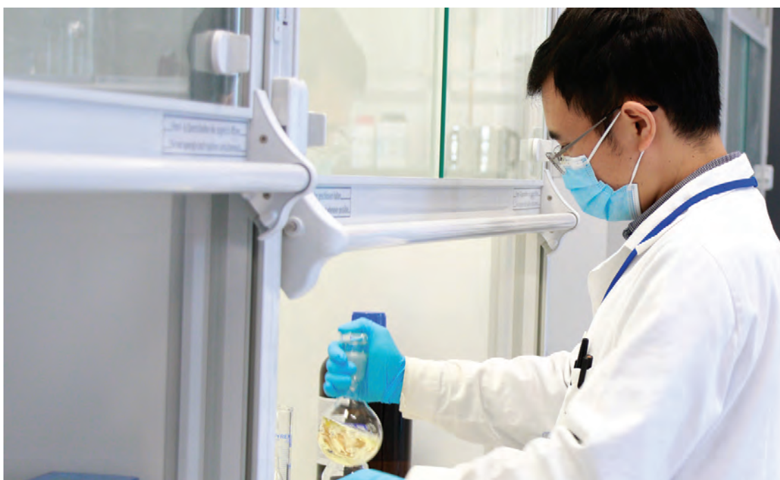
Sample preparation to verify the geographical origin and detect the adulteration of honey by measuring the ratio of stable isotopes of hydrogen ( \delta^2\text{H} ) in honey saccharides.
