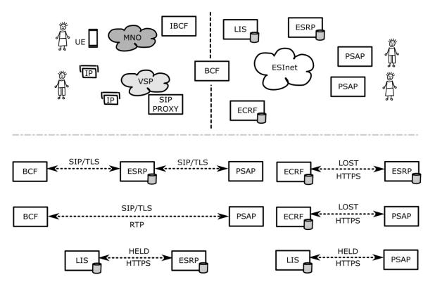
Figure 5: Functional elements and interfaces
