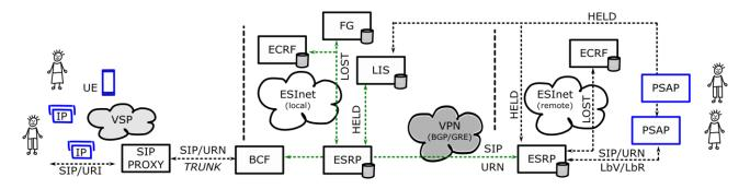
Figure 13: VSP Transatlantic Test Configuration
