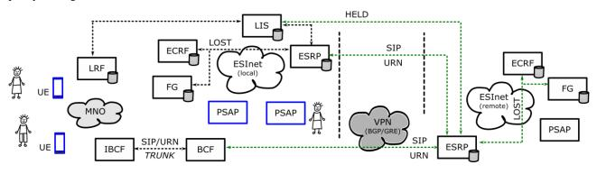
Figure 14: MNO Transatlantic Test Configuration
