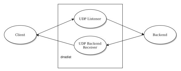
For UDP queries, dusdist stores the initial ID in a per-backend table called *IDState*. That ID then replaced by one derived from a counter before forwarding the query to the backend, to prevent duplicated IDs sent clients from making it to the backend. When the response is received, dusdist uses the ID sent by the backend to find the corresponding *IDState* and restores the initial ID, as well as some flags if needed, before sending the response to the client.
