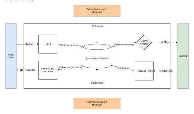
The following code shows a very simple example that forwards queries and responses to an external component over a unix network socket, and resumes them when it gets an answer from the external component.
