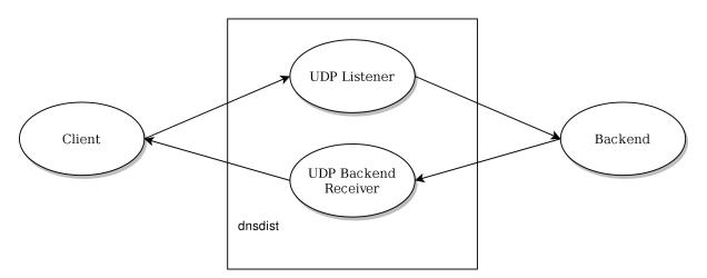
**dnsdist** design choices mean that the processing of UDP and DNS over HTTPS queries is done by only one thread per local bind (per addLocal(), addDNSCryptLocal() and addDOHLocal() directive).
