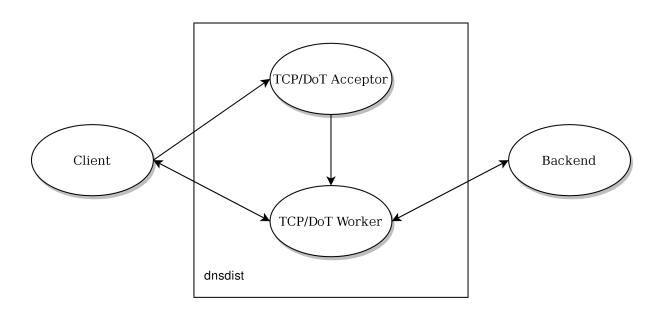
1000 (10000 on Linux since 1.6.0). Note that the size of the internal pipe used to distribute queries might need to be increased as well, using <code>setTCPInternalPipeBufferSize()</code>. Any value larger than 0 will cause new connections to be dropped if there are already too many queued.
