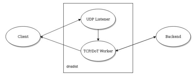
In that case the response will be sent back, directly by the TCP worker, over UDP, instead of being passed back to the UDP responder thread.
