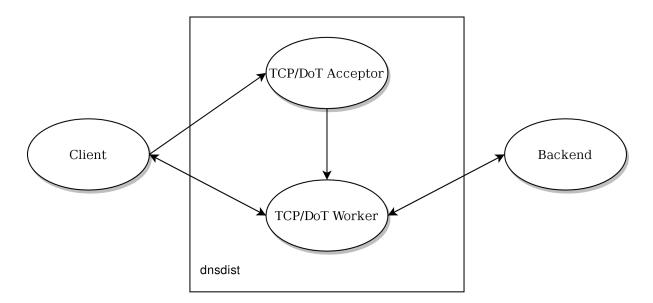
For TCP and DoT, a single thread is created for each <code>addLocal()</code> and <code>addTLSLocal()</code> directive, listening to the incoming TCP sockets, accepting new connections and distributing them over a pipe to the TCP worker threads. These threads handle both the TCP connection with the client and the one with the backend.
