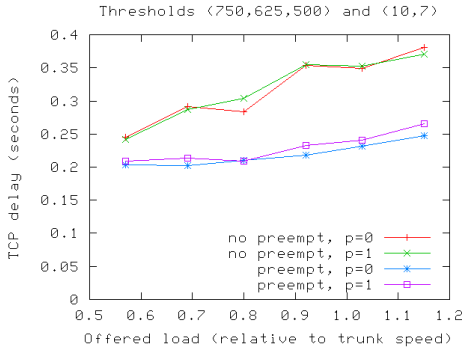
Fig. 7. Simulation results showing impact of CQ-ACM on delay in mixed traffic.
